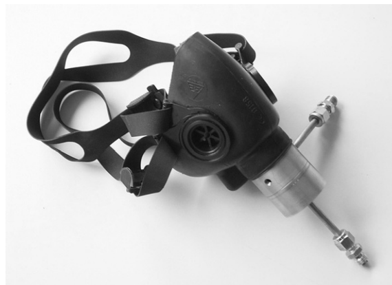
Figure 4. Picture of the breath mask for online exhaled air measurements.
